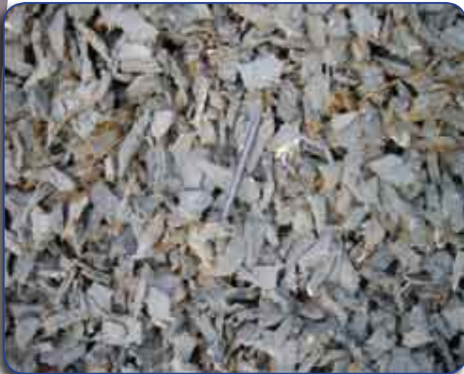
TDF particulate with bead wire removed Photo courtesy of Terry Gray, TAG
