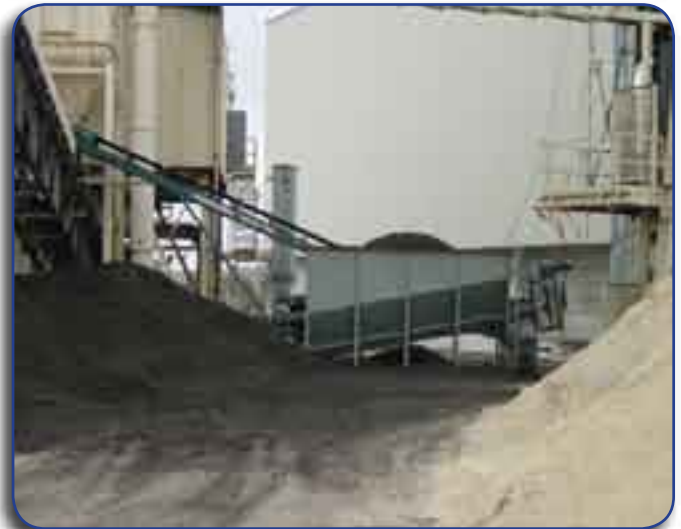
Metering system to introduce TDF into wood mixture before processing Photo courtesy of Terry Gray, TAG
