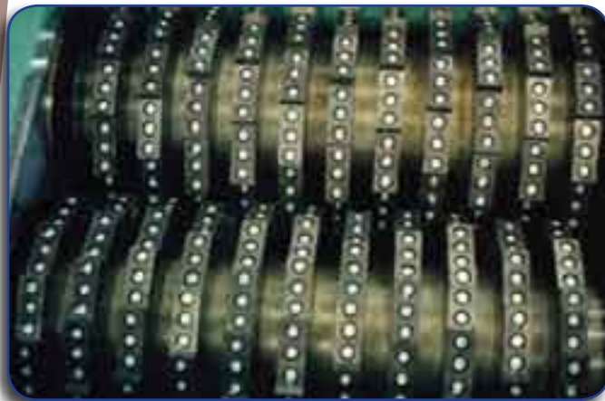
"Detachable knife" type shredder Photo courtesy of Columbus McKinnon Corporation, Sarasota, FL
