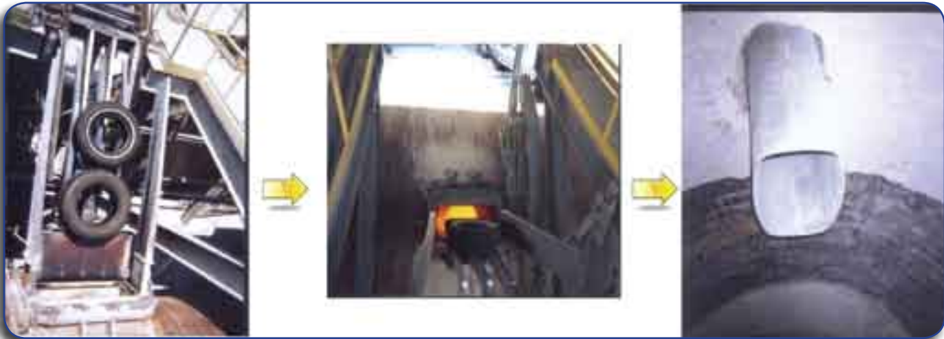
Exhibit 4-2. Mid-kiln injection Source: North Texas Cement
