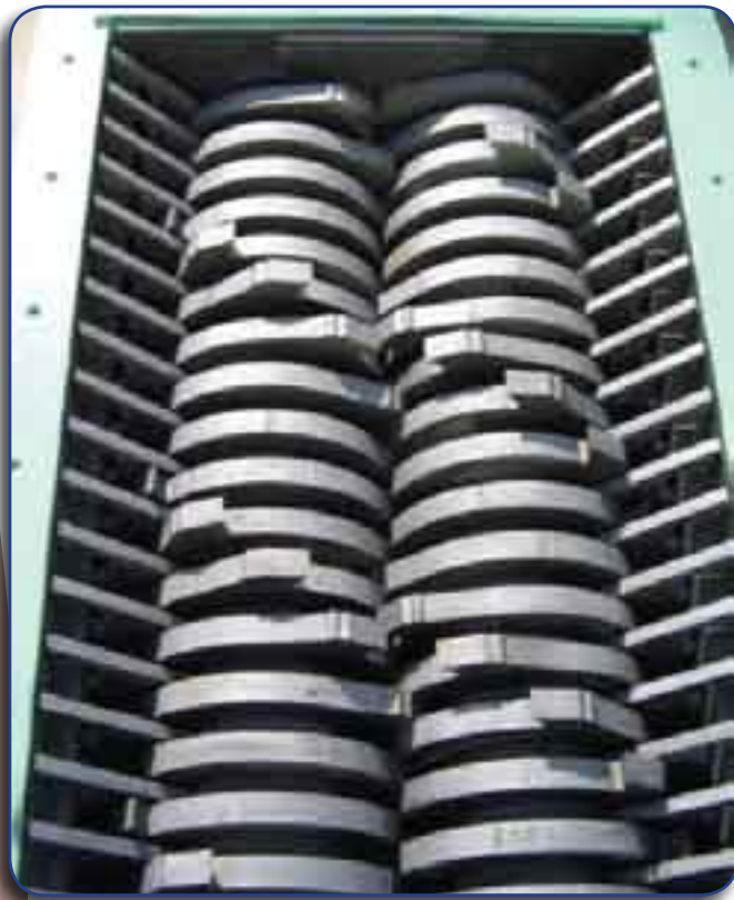
"Hook shear" type shredder Photo courtesy of Granutech Saturn Systems Corporation, Dallas, TX
